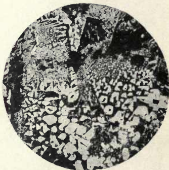
4.- Orthoclase. Ord. L. Showing alteration and intergrowth with quartz.
